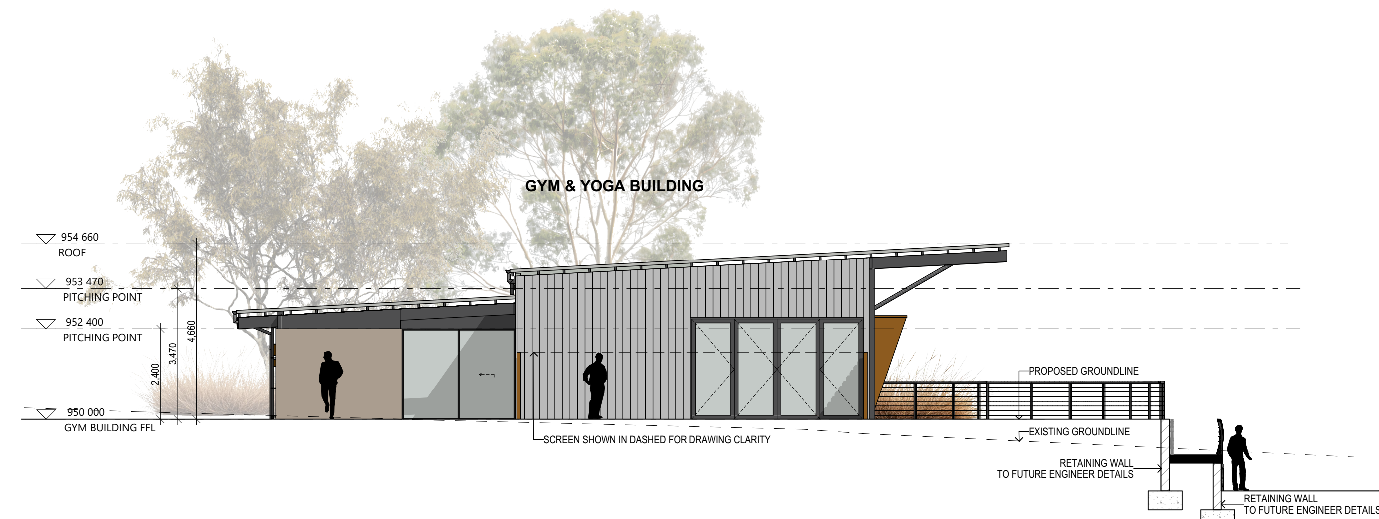
GYM BUILDING NORTH EAST ELEVATION 1:100
